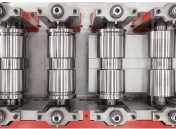
Answering to our customer's need, DIMECO offers the possibility of supplying the necessary set of rolls, in order to obtain different profiles in the existing rollforming machines.
