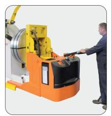
Step N°3 Then the operator can place the coil on the decoiler as simply as it puts a pallet on a palette rack.
