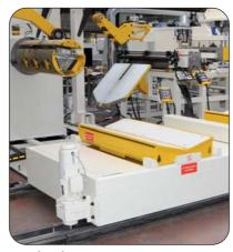
*Multi-Coil®* 4x10 tons, for moveable decoiler
