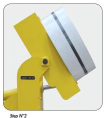
coil revolution by hydraulic cylinder.
