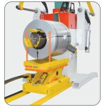
Step N°3 loading coil on the decoiler mandrel.
