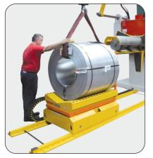
Step N°1 Coil drop by travelling crane or forklift while the line operates.
