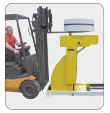
Step N°1 coil loading on the Tiltmatic® by a forklift truck.
