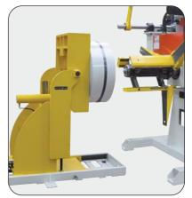
Positionning of the coil in the core axis
