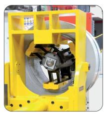
Step N°3 Translation of Tiltmatic® and mandrel expansion. Once the mandrel is expanded, the Tiltmatic® can be moved back in order to be released from the coil.
