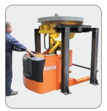
Step N°1 coil pick-up by the mobile Tiltmatic® on the storage rack.
