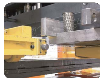
Bayonet-type coupling system. The tool is coupled onto the storage rack in concurrent operation time.
