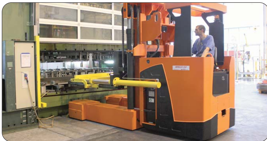
Tool loaded onto 1,000-tonne mechanical press
