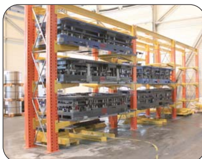
MAXI-CANTIBLOC®, total capacity: 37.5 tonnes (12.5 tonnes per tool)
