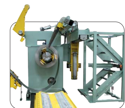
Coil-car with powered rolls
