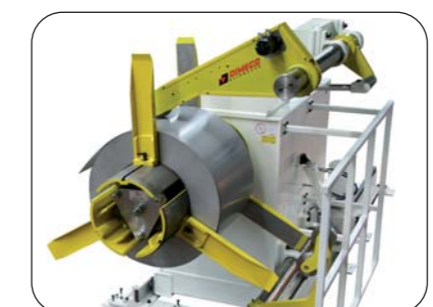
Motorized hydraulic pressure arm, two extra pressure arms to avoid self uncoiling when using HSLA
