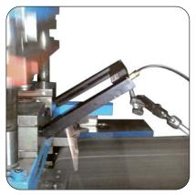
Frame sensor to check parts
