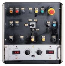
Load monitor integrated in the control cabinet
