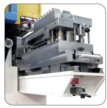
Tool combining cropping with end bending
