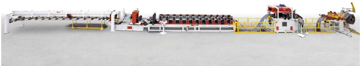
Flexipress in a flexible punching and rollforming line for highway safety barriers manufacturing.
