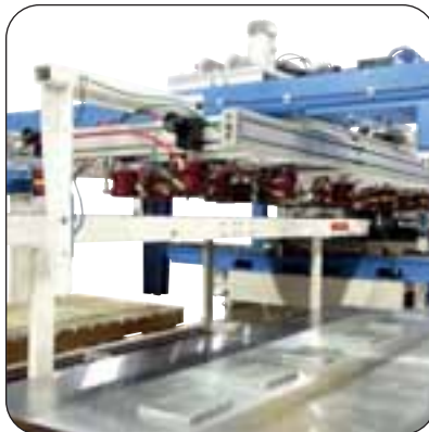
2D Stacker with magnetic suckers
