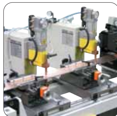
Spot welding of 2 superposed strips
