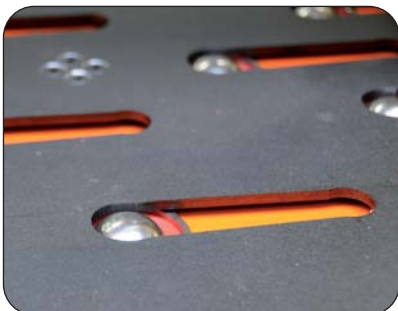
Active balls mean that the tool can be shifted easily
