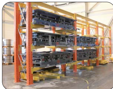
MAXI-CANTIBLOC®, total capacity: 37.5 tonnes (12.5 tonnes per tool)
