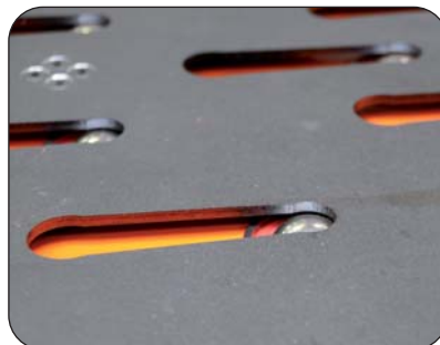
Inactive balls mean that the tool can be moved safely
