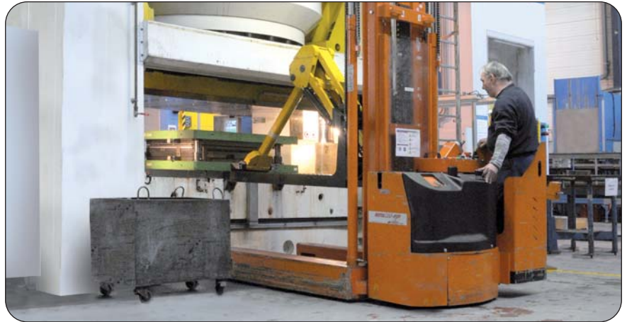
Tool-changeover on 6 000-tonne hydraulic press fitted with a Rotobloc-PSP magnetic tool-clamping system
