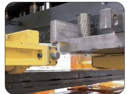
Bayonet-type coupling system. The tool is coupled onto the storage rack in concurrent operation time.
