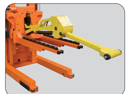
Truck fitted with a rotating apron (180° swing)
