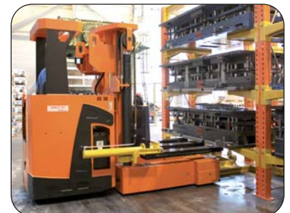
Tool taken up and stacked, without manual intervention
