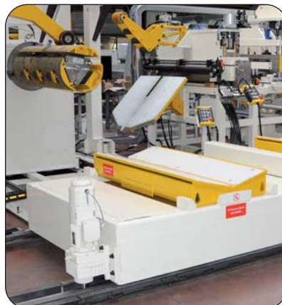
Multi-Coil® 4x10 tons, for moveable decoiler
