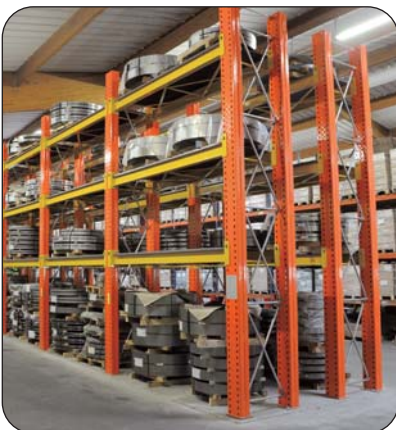
Extra-large coils holder 2 cells located back to back
