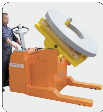
Step N°2 coil rotation on the mobile Tiltmatic®.
