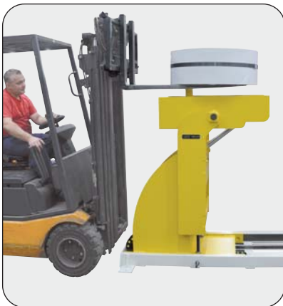
Step N°1 coil loading on the Tiltmatic® by a forklift truck.
