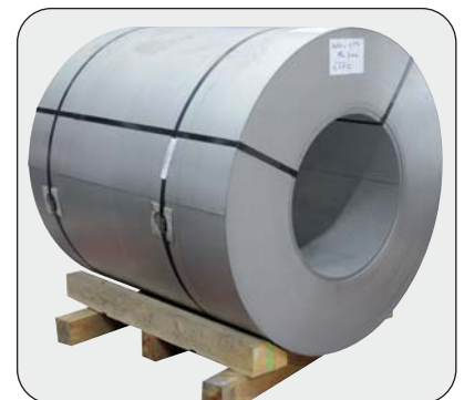
Large coils delivered with horizontal axis
