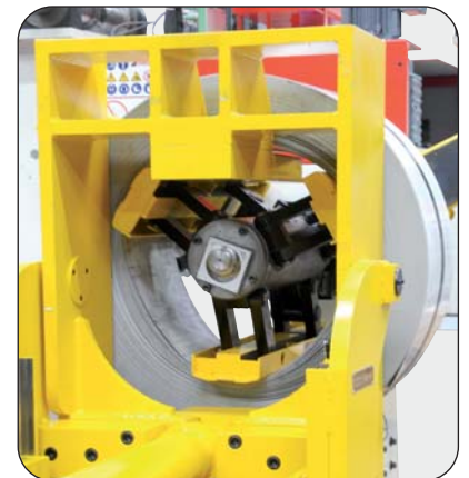
Step N°3 Translation of Tiltmatic® and mandrel expansion. Once the mandrel is expanded, the Tiltmatic® can be moved back in order to be released from the coil.
