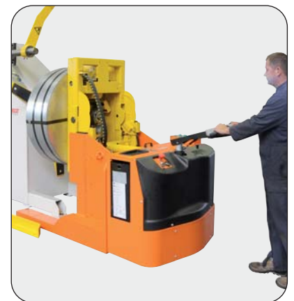
Step N°3 Then the operator can place the coil on the decoiler as simply as it puts a pallet on a pallet rack.
