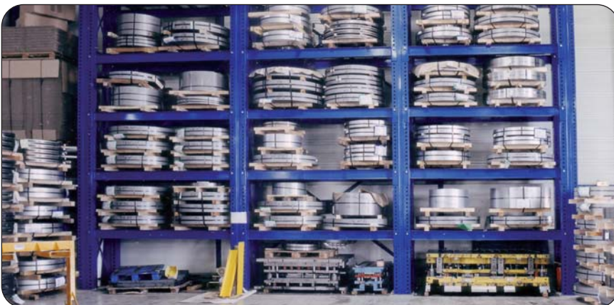
Extra-large coils holder 5x10 tons
