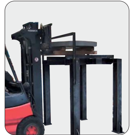
Before production change, the warehouse prepares the coil for next production by locating it into a specific cell in the storage rack.
