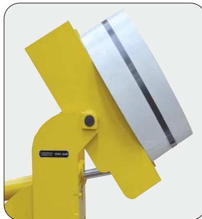
Step N°2 coil revolution by hydraulic cylinder.
