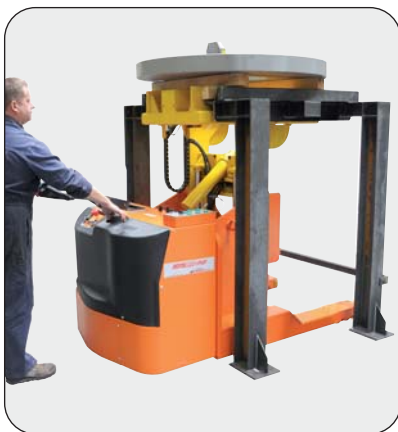
Step N°1 coil pick-up by the mobile Tiltmatic® on the storage rack.
